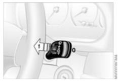
When the vehicle's lighting system is switched on, the headlamps will also be cleaned at reasonable intervals.
